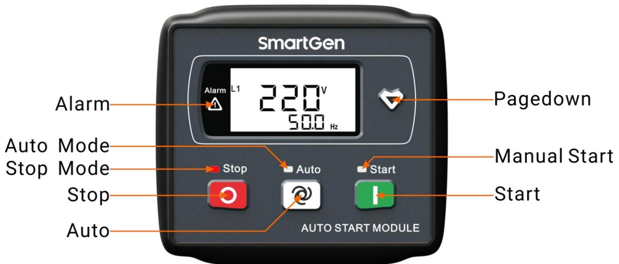
**Fig.1 HGM1790N Front Panel Indication**
