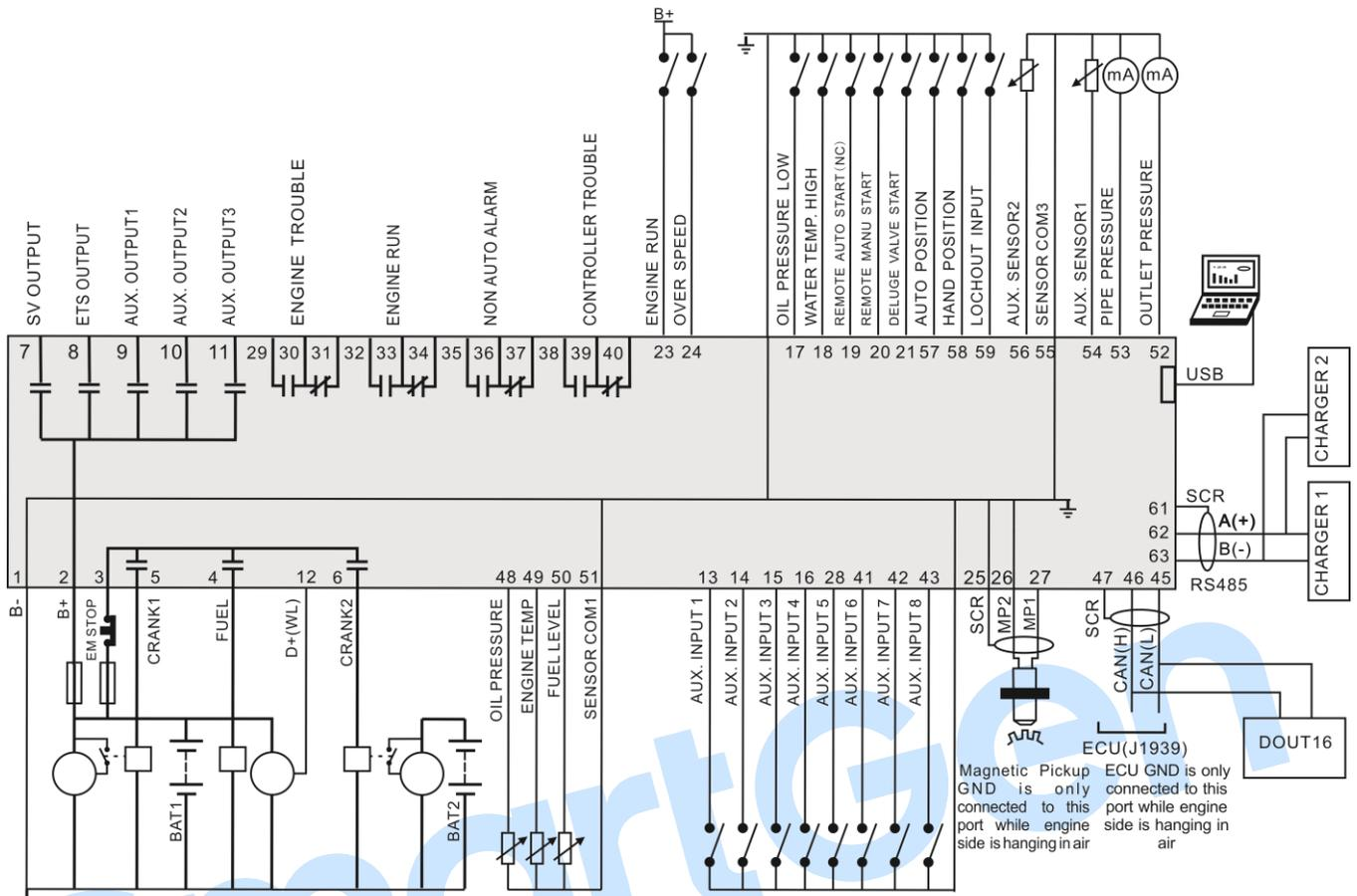
Fig.4 FPC915 Typical Application Diagram
