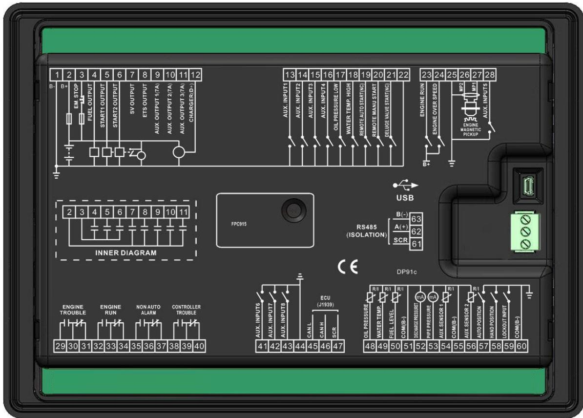
Fig.2 FPC915 Controller Back Panel
