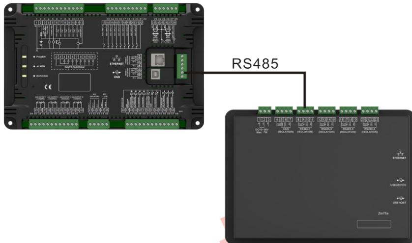
Fig.12-Wiring Diagram of Display Module and Master Control Module
