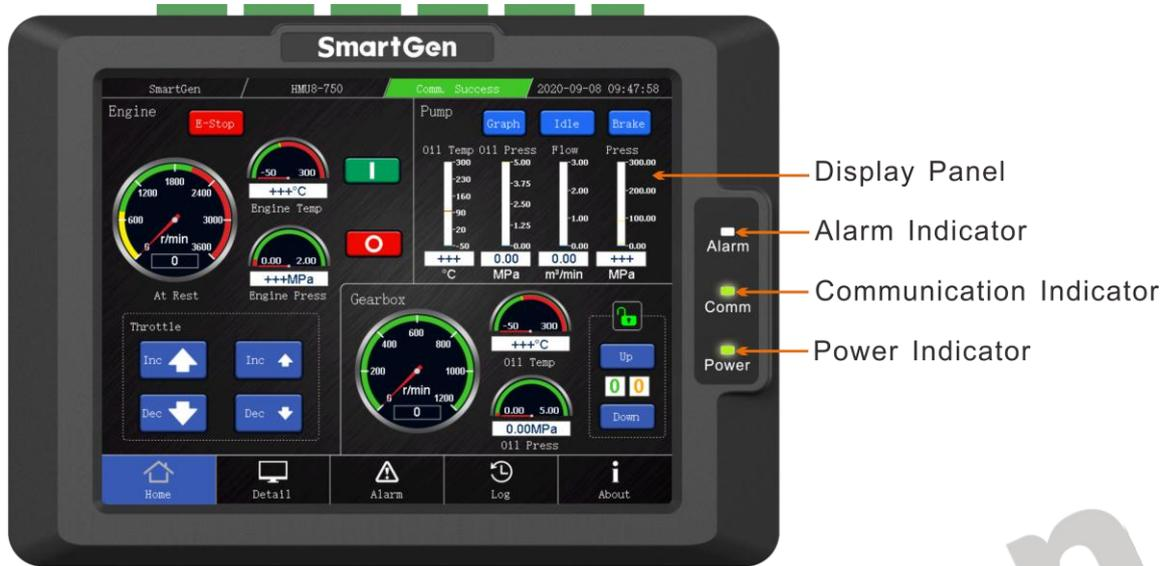
Fig.1-Display Module Front Panel
