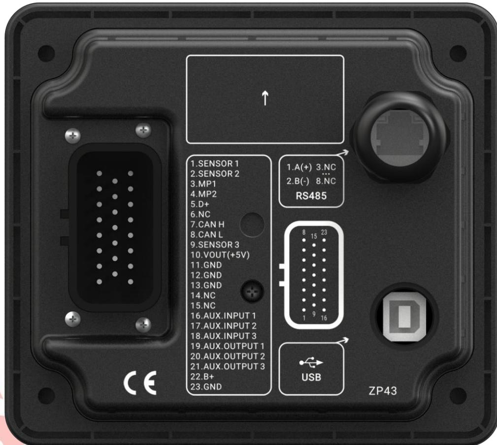
**Fig.2 – Controller Rear Panel**
