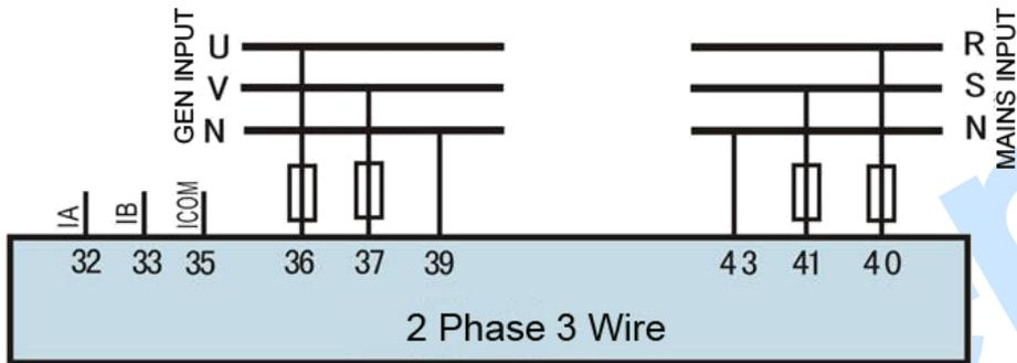
**Fig.8 2 Phase 3 Wire Connection Diagram**
