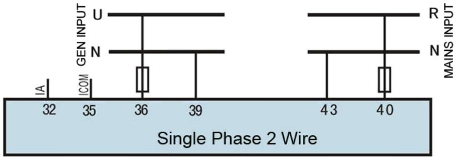
**Fig.7 Single Phase 2-Wire Connection Diagram**
