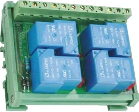
1. Fuel relay 30A, output voltage B+, coil power  $\leq 0.9W$
