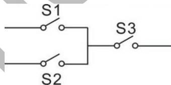
S1 or S2 is **TRUE**, while S3 is **TRUE**, Defined combination output is outputting;
