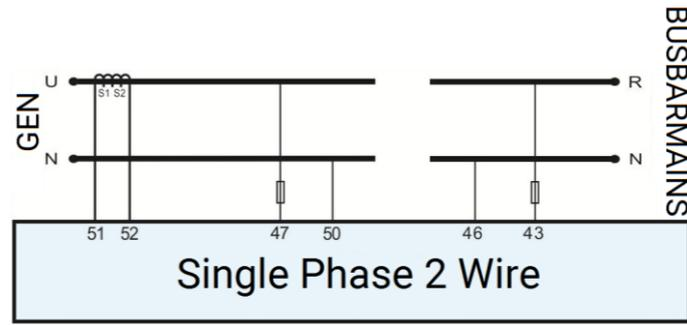
**Fig. 8 Single Phase 2-Wire Typical Application Diagram**
