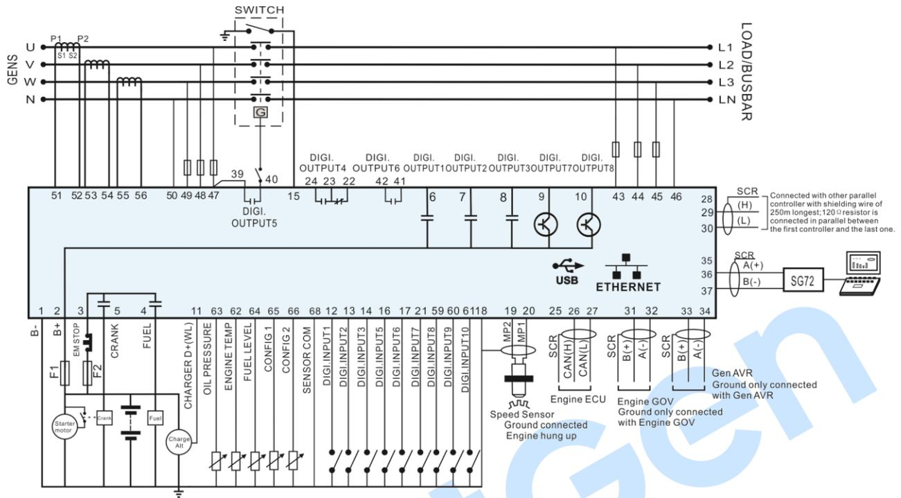
**Fig. 5 HGM9510N/HGM9530N 3-Phase 4-Wire Typical Application Diagram**
