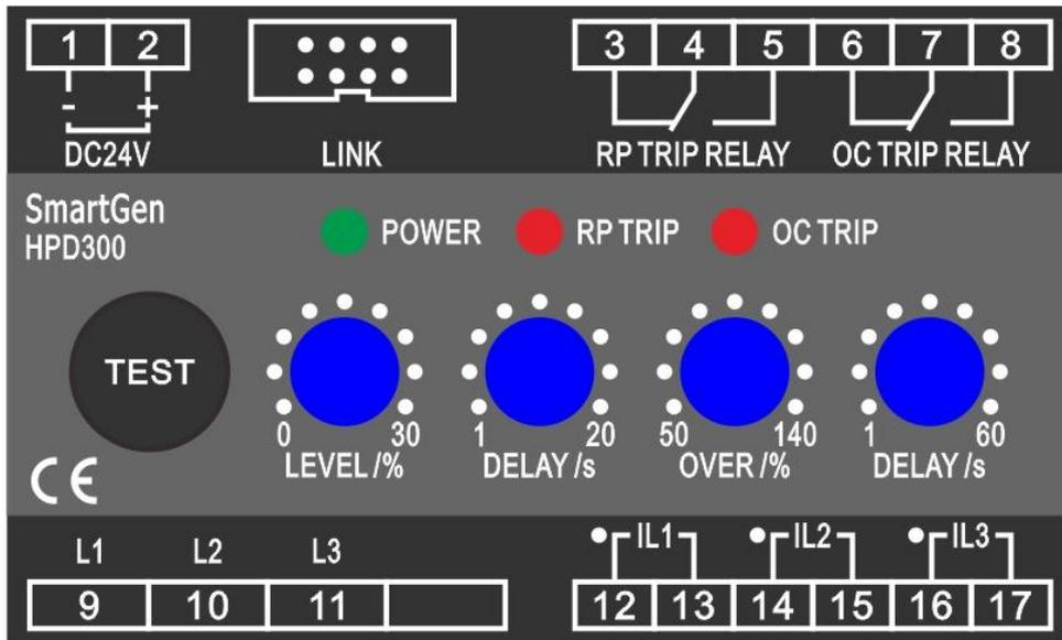
Fig.1 – Panel Drawing
