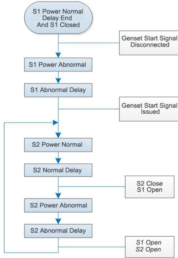
Fig. 8 Auto Transfer Non Restore Diagram (Mutual Backup Inactive)
