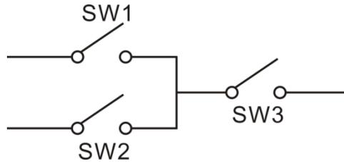
SW1 or SW2 is **TRUE**, and SW3 is **TRUE**, defined combination output is outputting;
