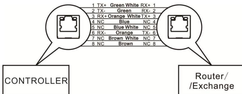
Fig. 13 Direct Connection Between Controller and Router
