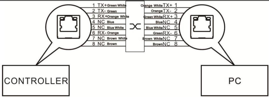
Fig. 14 Cross Connection Between Controller and PC
