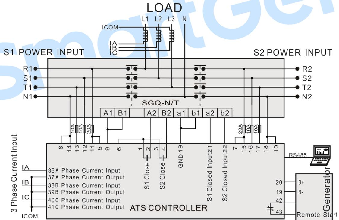
Fig. 19 SGQ-N/T Application Diagram
