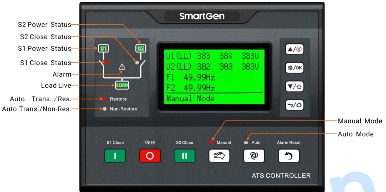
Fig. 2 Front Panel
