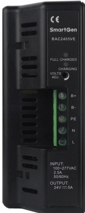
1. Connect terminals L and N to alternating voltage (100~277)V using BVR 1mm<sup>2</sup> multi-strand copper line.
