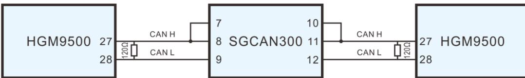
Fig. 5 – Typical Application Diagram of MSC1 and MSC2
