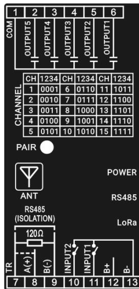
Fig.5 Mask Diagram
