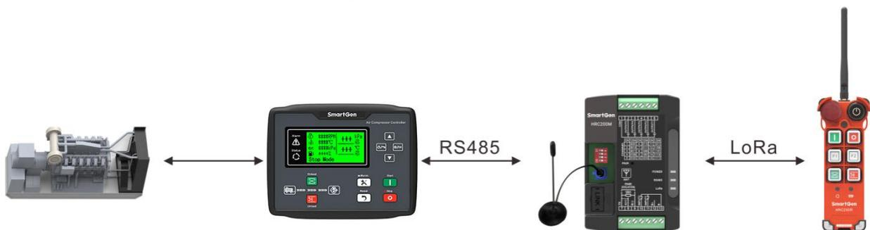
**Fig.7 HRC200 System Application Diagram**
