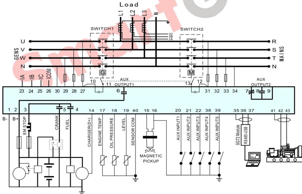
Fig.5 - HGM6120LT Typical Application Diagram
