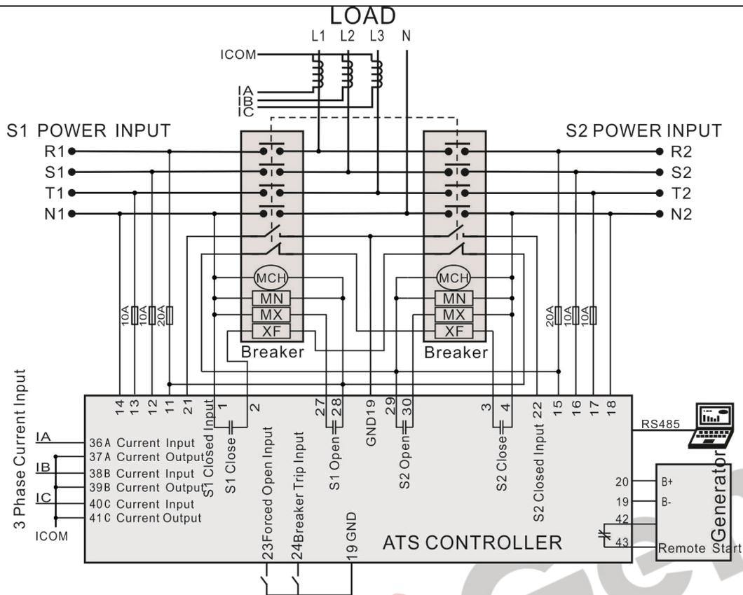
Fig. 27 Breaker Application Diagram
