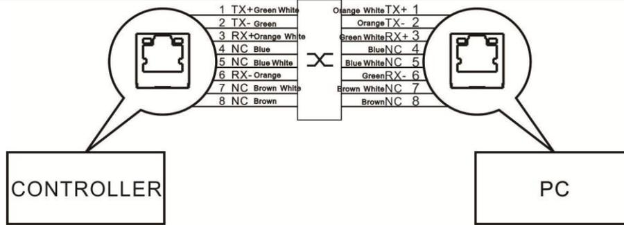
Fig. 17 Cross Connection Between Controller and PC
