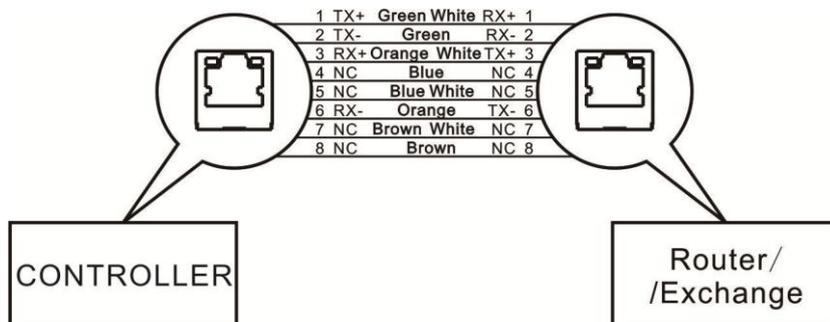
Fig. 16 Direct Connection Between Controller and Router
