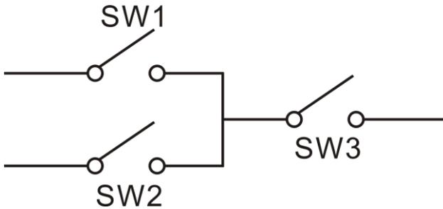
SW1 or SW2 is **TRUE**, while SW3 is **TRUE**, Defined combination output is active;
