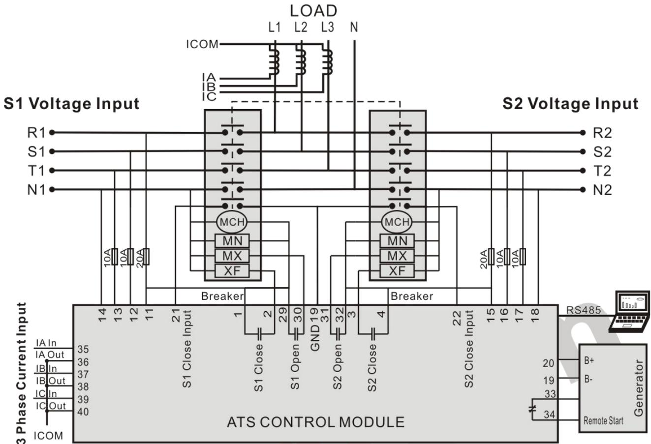
MCH: Stored Energy Motor; MN: Under Voltage Trip; MX: Open Relay; XF: Close Relay;
