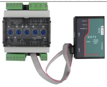
Fig.2 - PC Programming Connection
