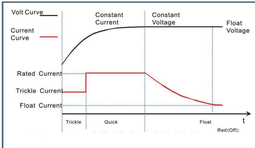
Charging is performed according to the battery charging characteristics using two-stage method.
