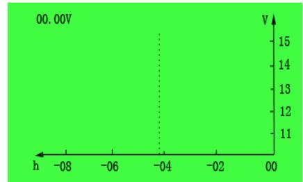
record. In curves interface, press
