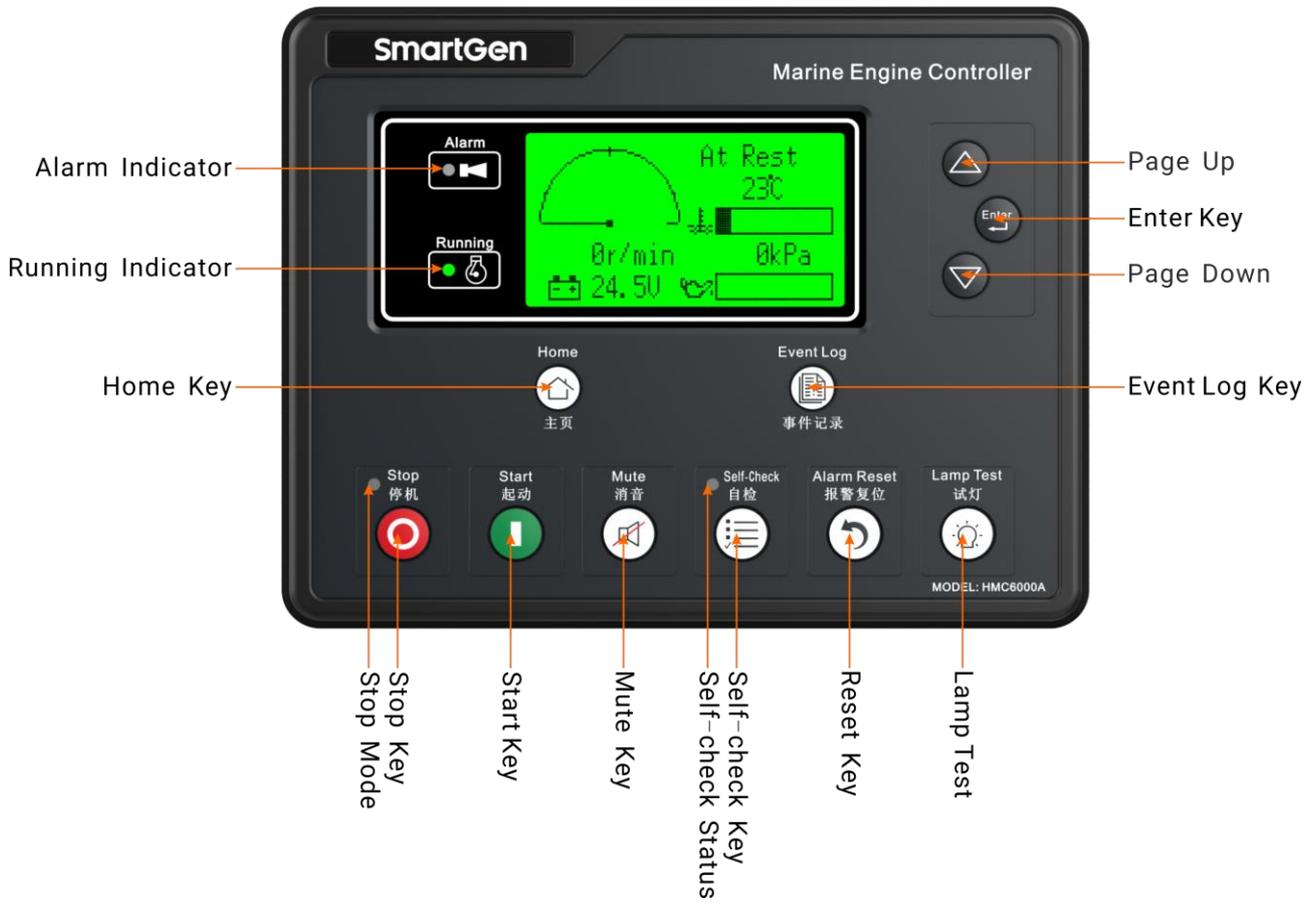
**Fig.1 HMC6000A Front Panel**
