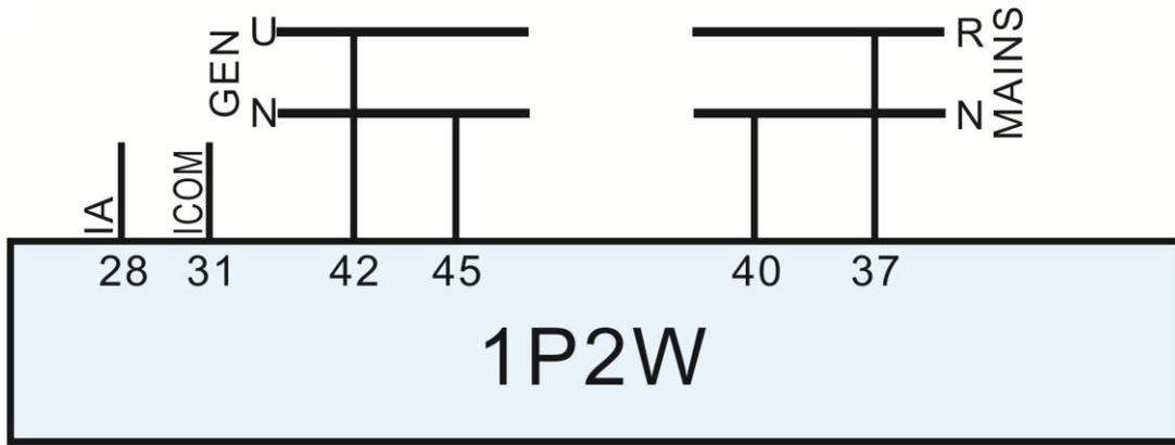
**Fig. 10 – Single Phase 2 Wire Diagram**
