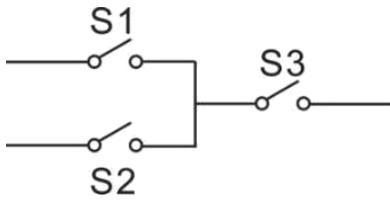
S1 or S2 is **TRUE**, while S3 is **TRUE**, custom combination output is outputting;
