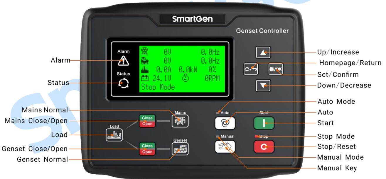
**Fig.2 – HGMS62D Front Panel Indication**
