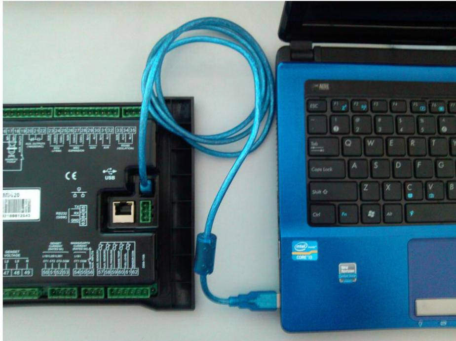
**Fig.12 USB Connection Method**
