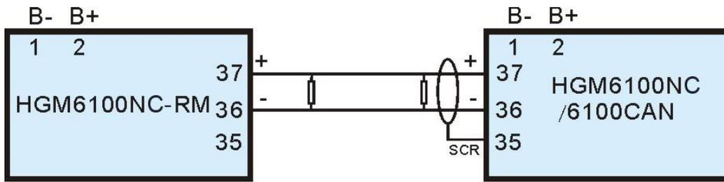
**Fig. 4 HGM6100NC-RM and HGM6100NC/CAN Typical Application Diagram**
