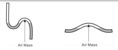
Fig. 4 - Incorrect Pipe Connection Methods
