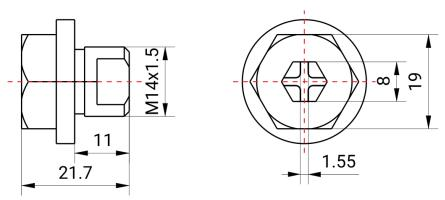
Fig.7 - Water Drain Valve
