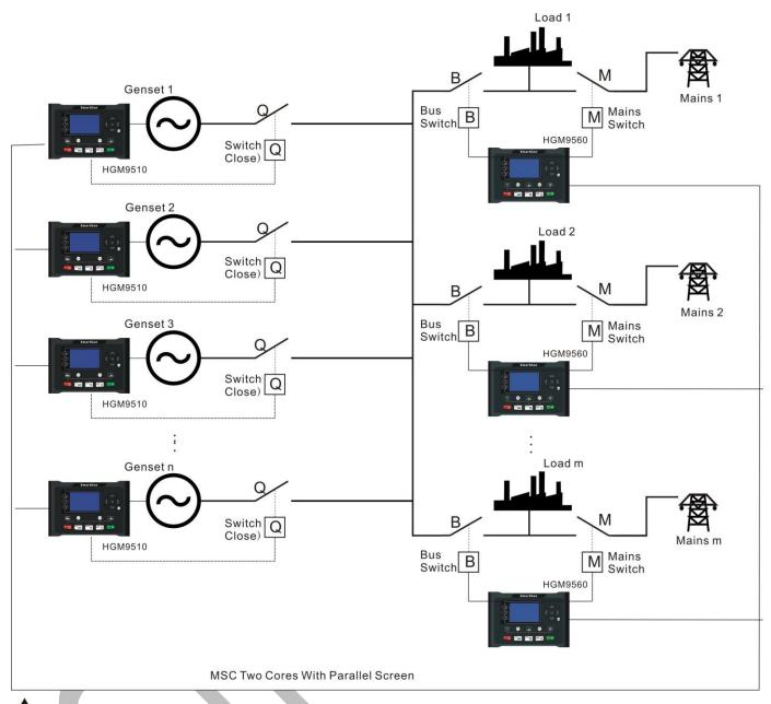
Note: Bus CT is important for multi set communication, so make sure that it is soundly connected.
