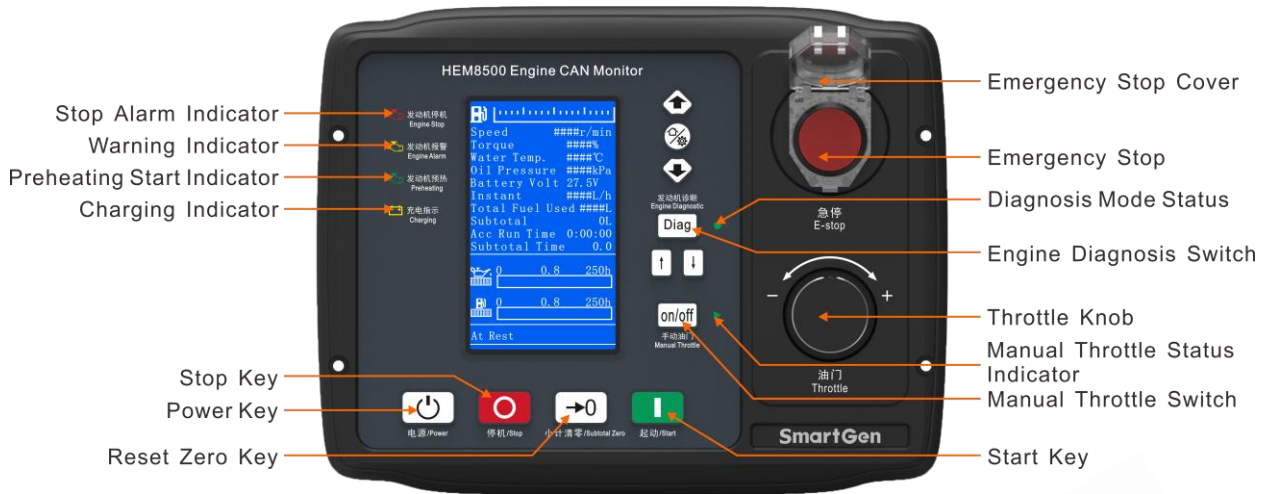
Fig. 1 HEM8500 Front Panel Indication
