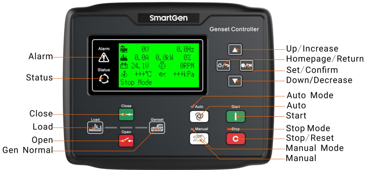
Fig.1 – HGM6110 (HGM6110N/NC/CAN) Front Panel Indication
