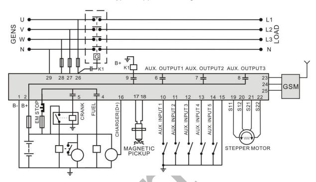
**CAUTION!** Expand relay with high capacity in start and fuel output is recommend.
