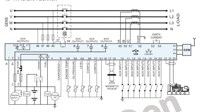
Fig.3 HGM8110N Typical Application Diagram
