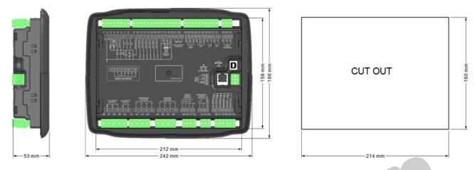
Fig.6 Overall Dimensions and Panel Cutout
