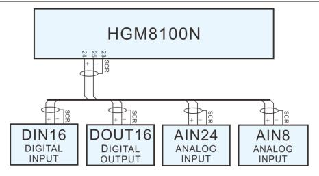
Fig.5 HGM8100N Expansion Module Typical Application Diagram
