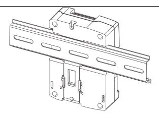
Fig.11 HRC200M Guide Rail Installation
