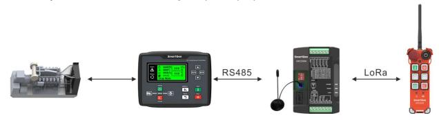
Fig.7 HRC200 System Application Diagram
