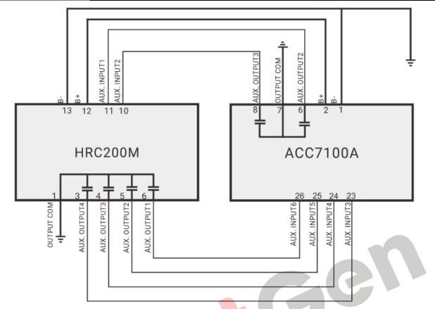
Fig.8 HRC200M Digital Control Application Diagram
